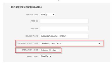
**Arduino Board Type**: Define the bootloarder/mcu type/ fuse setting during Sketch upload. **Operation Mode:** make sure it is in <u>Arduino Bridge</u> mode so the Bridge class for Arduino Yun works.
