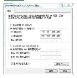
A fall back IP 172.31.255.254/255.255.255.252 is assigned to Yun Shield's LAN port so user can always access Yun Shield with this ip if their laptop has the IP 172.31.255.253/255.255.255.252.
