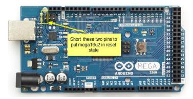
2) Add a "Mega2560 Yun" board type in the file: Arduino\hardware\arduino\avr\board.txt. as below and reopen the Arduino IDE:
