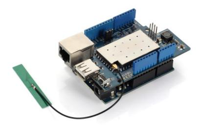
Basically, Yun Shield + Leonardo equally to the official Arduino Yun, but Yun Shield is more flexible because it can work with other Arduino board such as Uno, Duemilanove, Mega etc. And Yun Shield uses external wifi antenna which provides stability and possibility for various environments.
