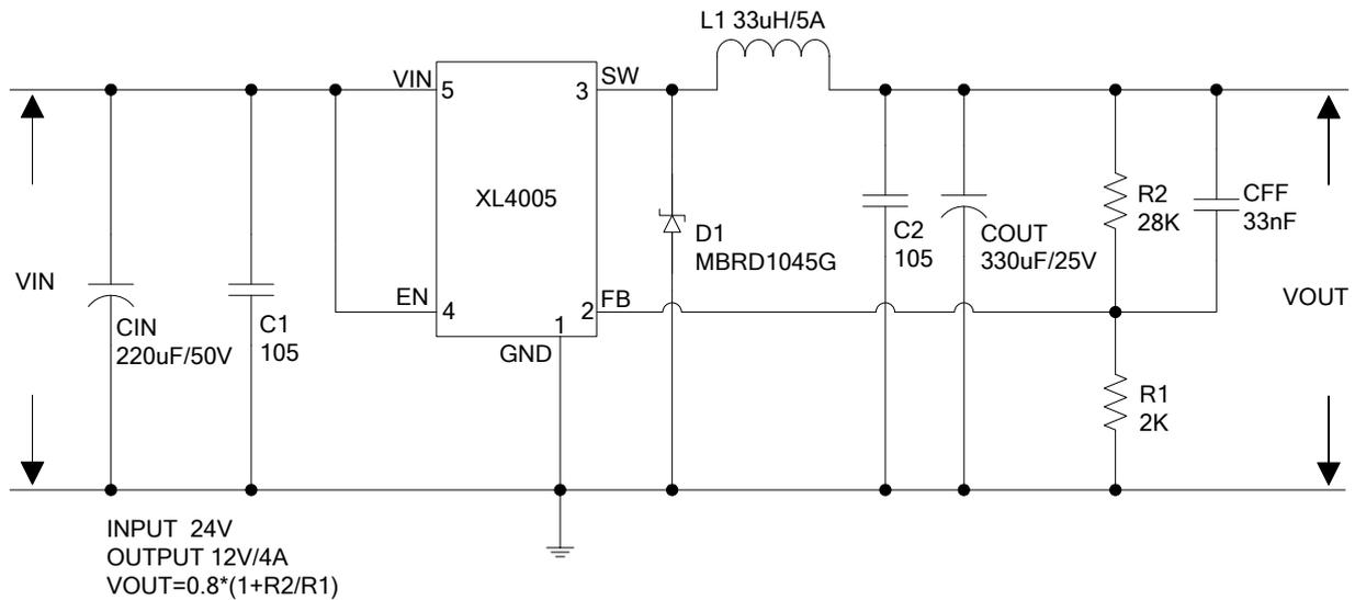
Figure6. XL4005 System Parameters Test Circuit (24V ~ 12V/4A)
