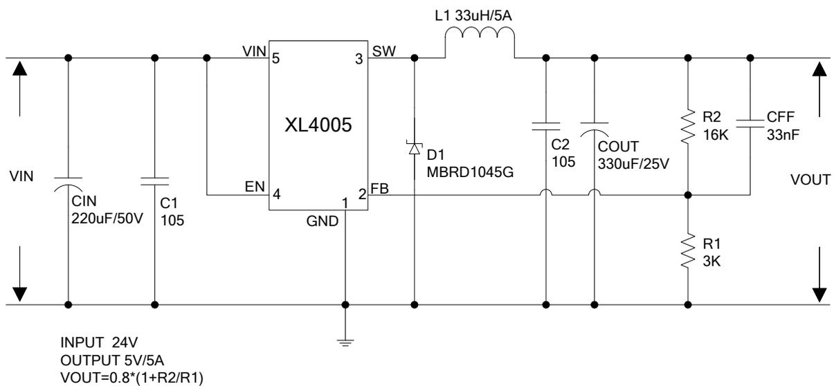
Figure7. XL4005 System Parameters Test Circuit (24V ~ 5V/5A)
