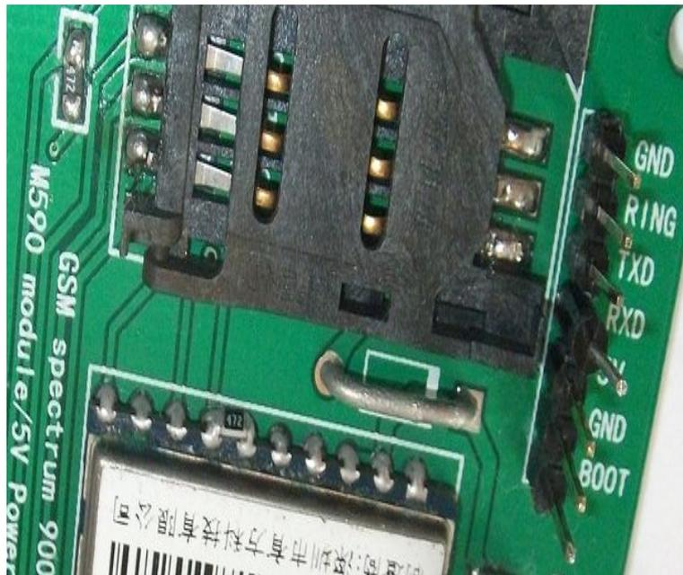
Figure 34 Top view of the M590E V1 module
