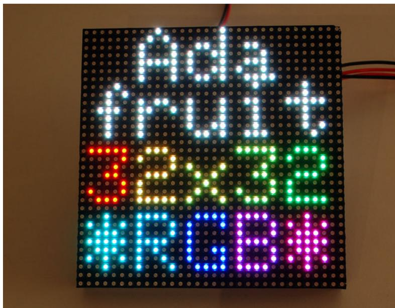
These panels require 12 or 13 digital pins (6 bit data, 6 or 7 bit control) and a good 5V power supply, up to 2A per panel (when on full white). We suggest our 2A regulated 5V adapter and either a terminal block DC jack, or solder a jack from our DC extension cord. Please read the
