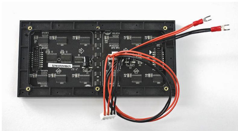
The spades at the opposite end of this power cable can be screwed into a 2.1mm terminal block adapter. Works nicely! Don't allow the exposed connectors to contact metal though...you may want to cover this with heat-shrink tube or electrical tape.
