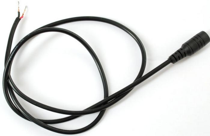
Solder both pins correctly to the power port. Make sure you get this right because there is no protection diode!
