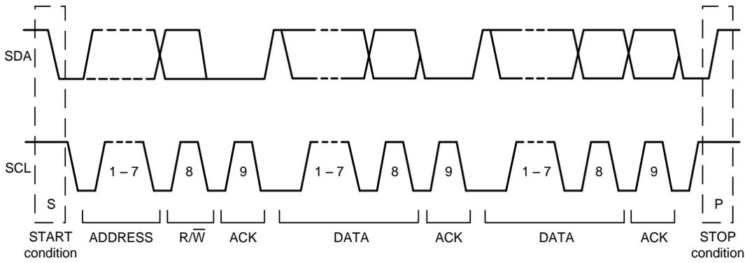
**Figure 11: Complete I<sup>2</sup>C Data Transfer**
