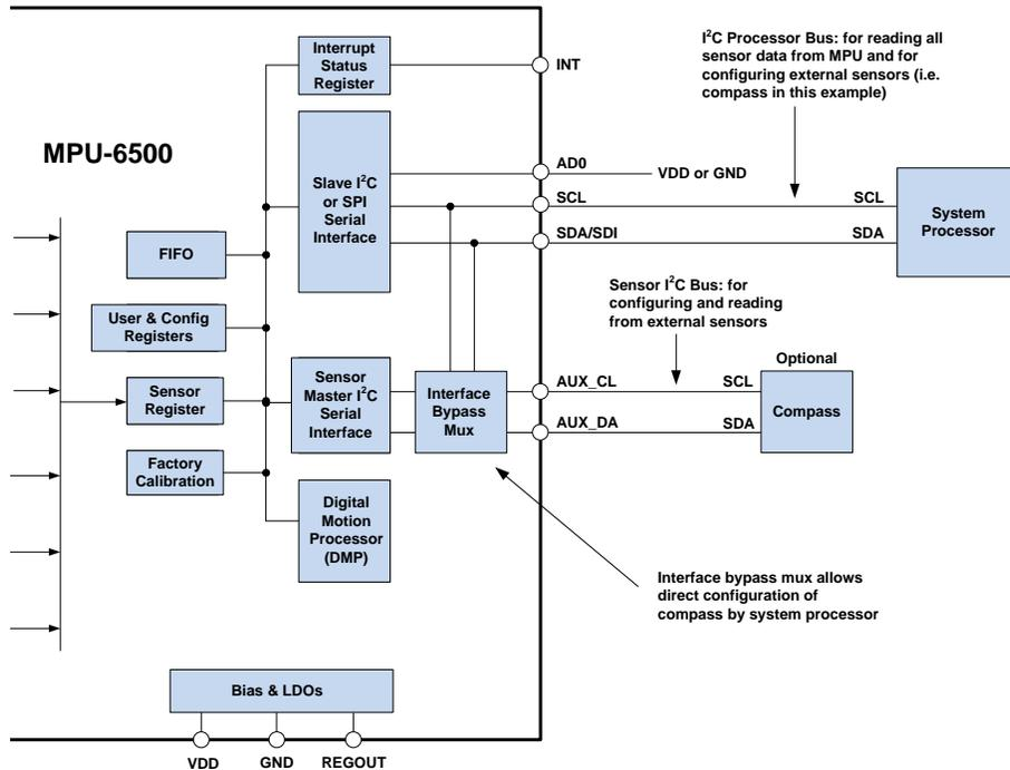
**Figure 6: MPU-6500 Solution Using I<sup>2</sup>C Interface**
