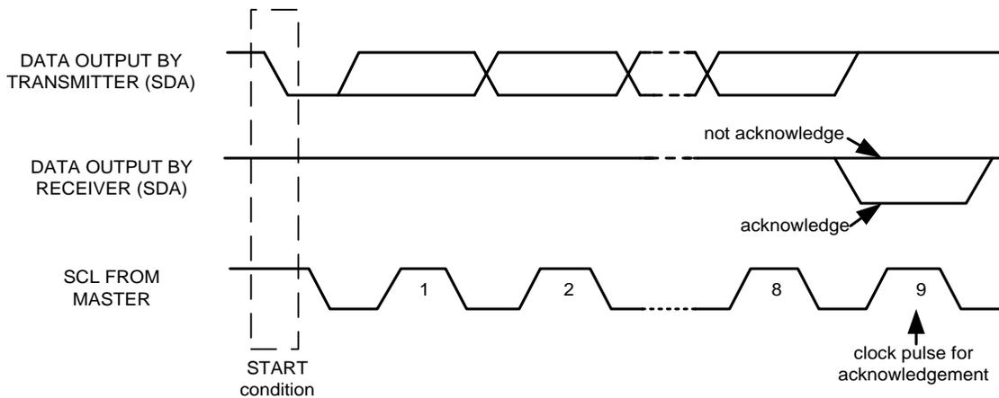
**Figure 10: Acknowledge on the I<sup>2</sup>C Bus**
