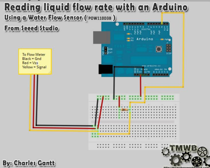
Once you have it wired up you will need to upload the following code to your Seeeduino. Once it is uploaded and you have some fluid flowing through the Water Flow Sensor, you can open the serial monitor and it will display the flow rate, refreshing every second.
