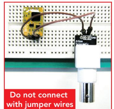
Do not connect with jumper wires
