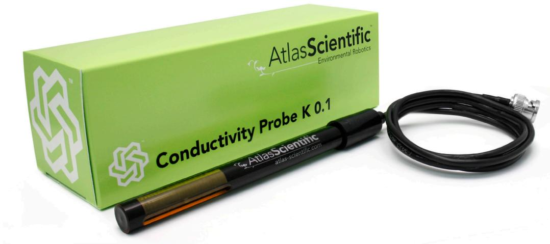
This Atlas Scientific conductivity probe, has a cell constant of **K 0.1**. When this conductivity probe is connected to an Atlas Scientific EZO™ conductivity circuit, it has a range of **0.5  $\mu\text{S}/\text{cm}$  to 50,000  $\mu\text{S}/\text{cm}$** .
