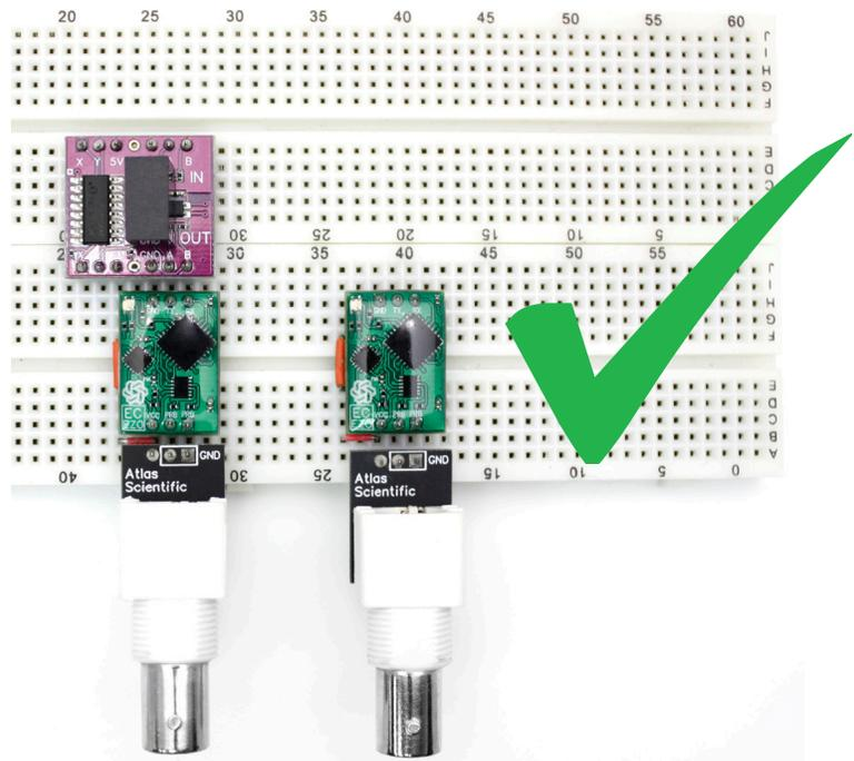
To correct this problem the power and data lines need to be electrically isolated. There is no one single method of doing this. This is just one of many ways to do so.
