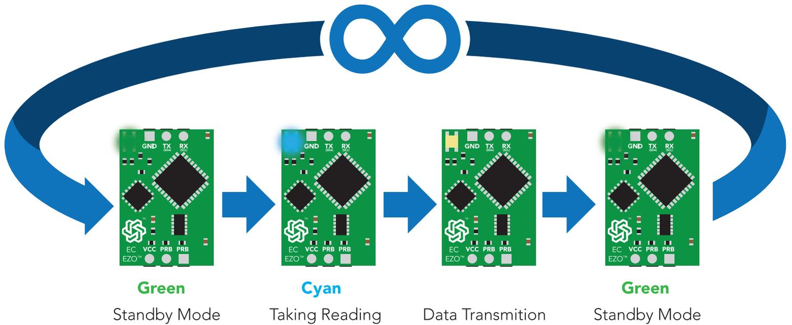
This is the LED pattern for Continuous Mode (which is the default state)
