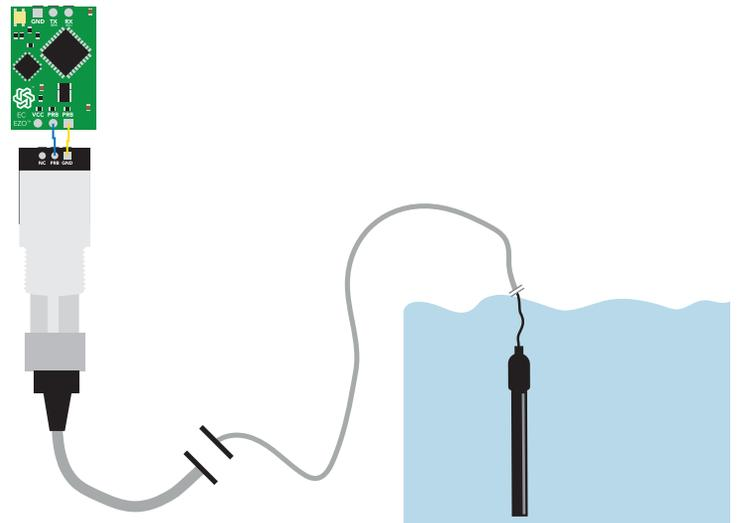
When reading from two conductivity circuits, it is strongly recommended that one of them is electrically isolated
