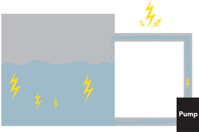
When electrical noise is interfering with the Conductivity readings it is common to see rapidly fluctuating readings or readings that are consistently off. To verify that electrical noise is causing inaccurate readings place the Conductivity probe in a cup of water by itself. The readings should stabilize quickly, confirming that electrical noise was the issue.
