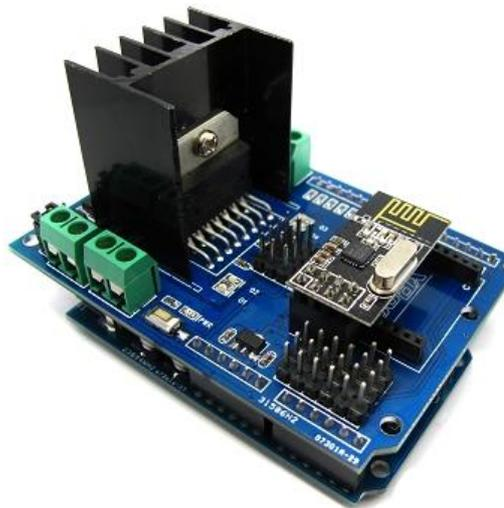
MotoMama is an H-Bridge motor driver shield based on ST L298N chip. It is a high voltage, high current dual full-bridge driver which designed to accept standard TTL logic levels and drive inductive loads such as relays, solenoids, DC motor and stepping motors. MotoMama is designed to be easy with other sensors or wireless modules.
