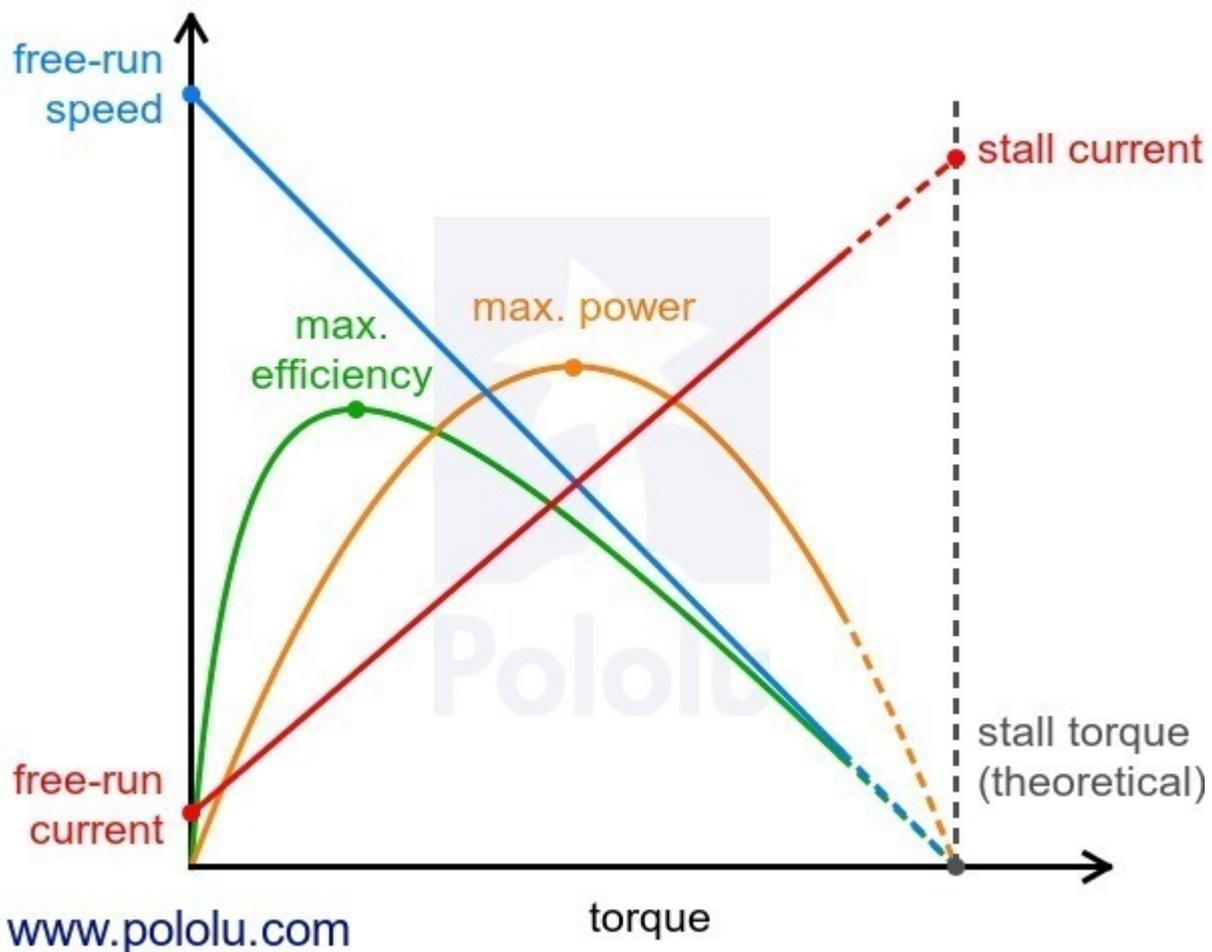
The current and speed curves are approximately linear, and the product pages for our motors provide the approximate end points for these lines: (0 torque, no-load current) and (stall torque, stall current) for the red line, and (0 torque, no-load speed) and (stall torque, 0 speed) for the blue line.
