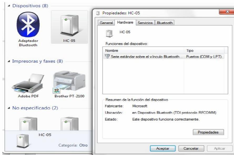
Open a serial terminal and select the serial COM x port number that assigned Windows to Bluetooth Module.
