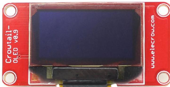
The Crowtail- OLED is constructed with 128 x 64 dot matrix OLED module. Users can display characters& pictures on this small screen.
