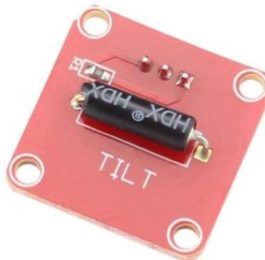
The Crowtail- Tilt Switch is a sensor to detect the station of forwards. It outputs logic LOW in Horizontal direction and logic HIGH in Vertical direction.
