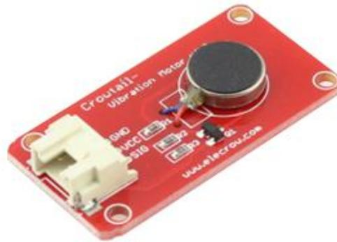
The vibration modules vibrates when it activated by signal logic HIGH, like the vibration of a phone. This module is consist of a permanent magnet coreless DC motor.
