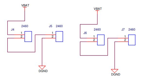
Figure 4. Battery Holder Configuration
