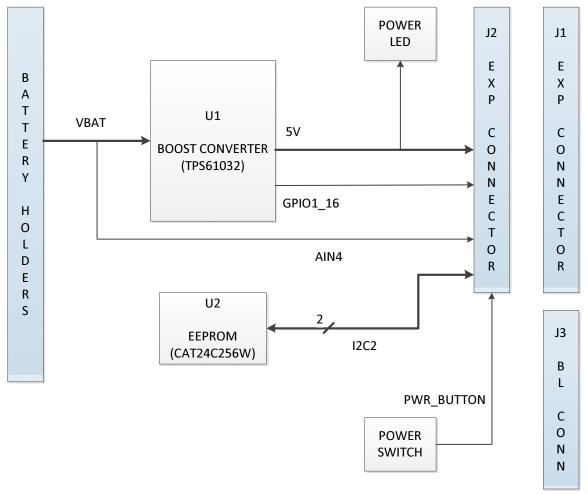
Figure 3. BeagleBone Battery Cape High Level Block Diagram
