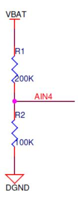
Figure 5. Battery voltage level divider
