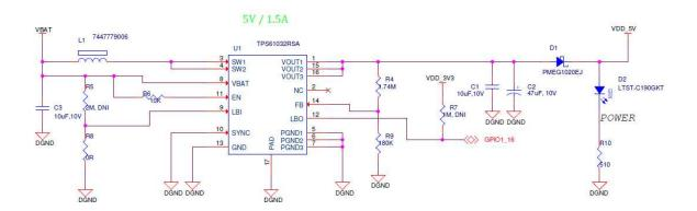
Figure 6. Boost converter circuit
