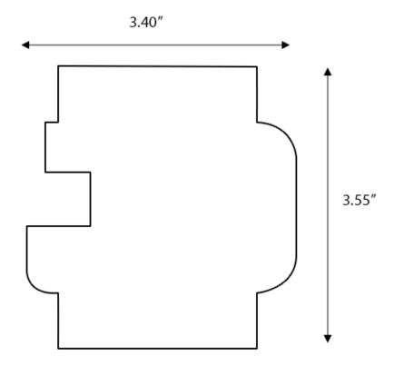
Figure 8. BeagleBone LCD3 Cape Dimensions Drawing
