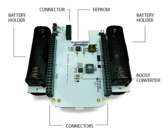
Figure 2. Battery Cape key components
