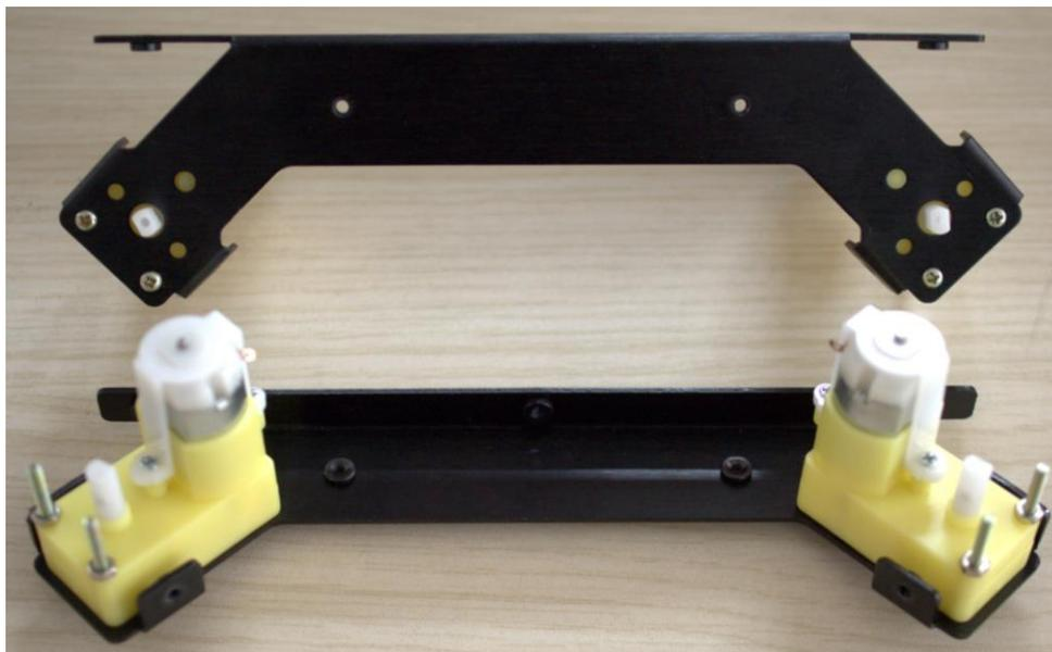
**2. To fix the connecting rod on the edge of the side-panel and install wheels**
