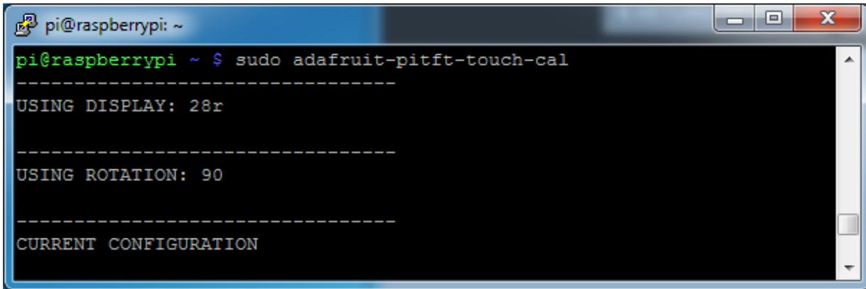
A terminal window titled 'pi@raspberrypi: ~' showing the execution of the 'sudo adafruit-pitft-touch-cal' command. The output is as follows:
