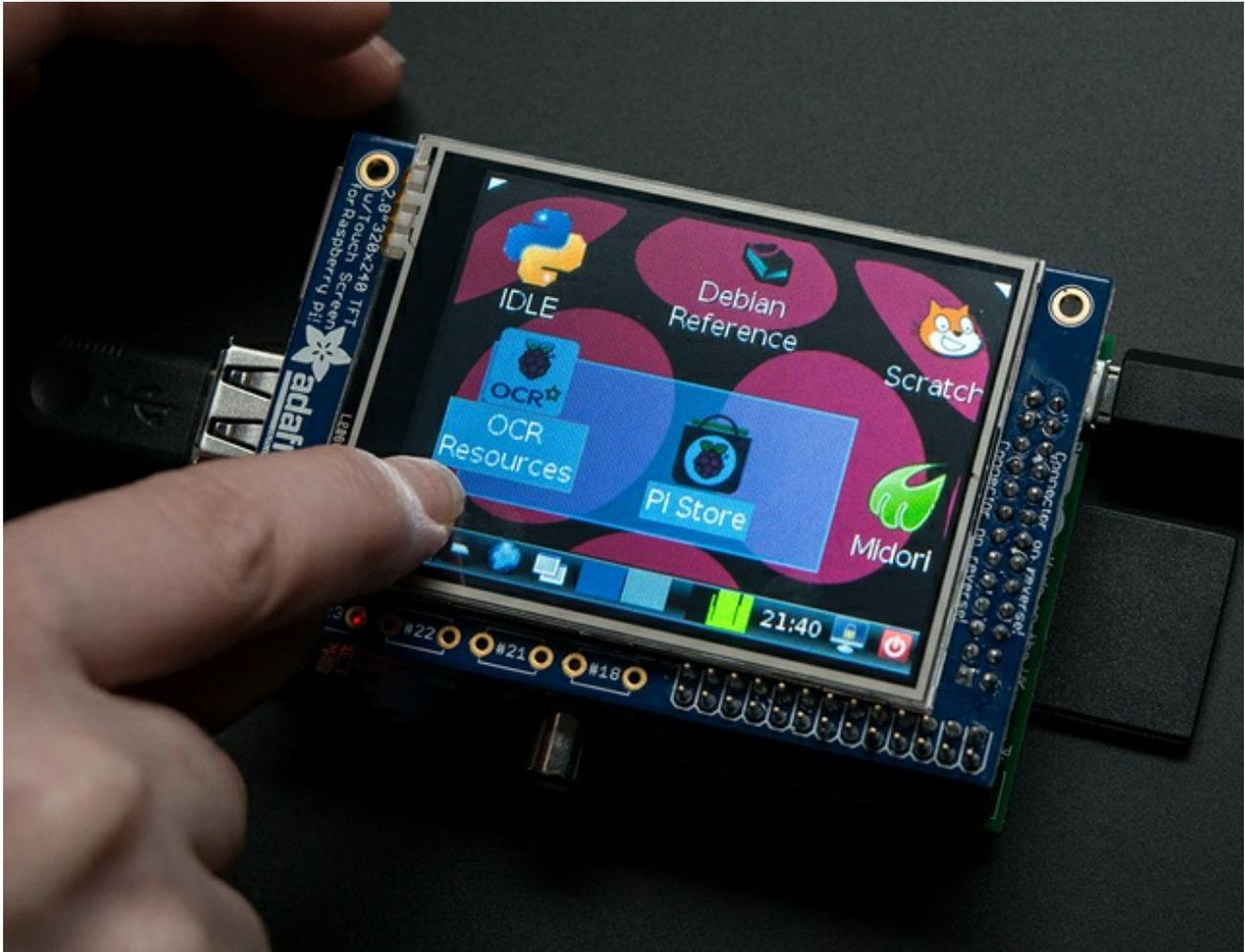
Is this not the cutest little display for the Raspberry Pi? It features a 2.8" display with 320x240 16-bit color pixels and a resistive touch overlay. The plate uses the high speed SPI interface on the Pi and can use the mini display as a console, X window port, displaying images or video etc. Best of all it plugs right in on top!
