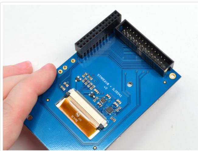
If you want to attach an Adafruit Cobbler or similar, you can solder in the optional 2x13 IDC on the **bottom** of the screen as shown here. This will keep the top side clean and flat. Solder in all 26 pins
