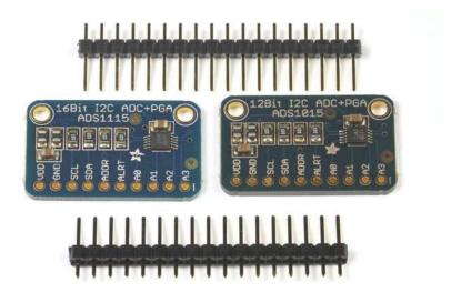
The ADS1115 and ADS1015 4-channel breakout boards are perfect for adding high-resolution analog to digital conversion to any microprocessor-based project. These boards can run with power and logic signals between 2v to 5v, so they are compatible with all common 3.3v and 5v processors. As many of 4 of these boards can be controlled from the same 2-wire I2C bus, giving you up to 16 single-ended or 8 differential channels. A programmable gain amplifier provides up to x16 gain for small signals.
