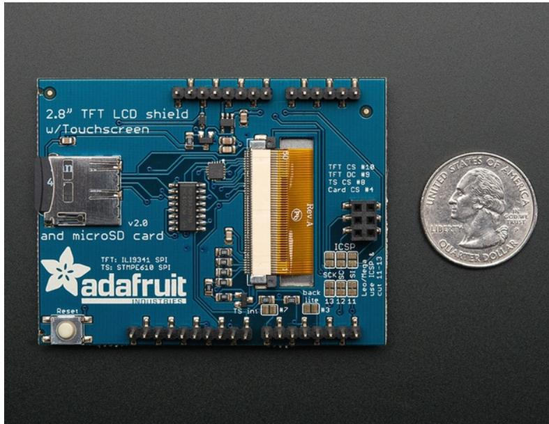
**The shield is fully assembled, tested and ready to go. No wiring, no soldering! Simply plug it in and load up our library - you'll have it running in under 10 minutes!** Works best with any classic Arduino (UNO/Duemilanove/Diecimila). Solder three jumpers and you can use it at full speed on a Leonardo or Mega as well.
