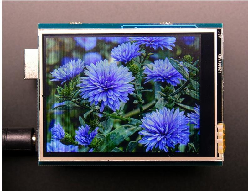
To make new bitmaps, make sure they are less than 240 by 320 pixels and save them in **24-bit BMP format!** They must be in 24-bit format, even if they are not 24-bit color as that is the easiest format for the Arduino. You can rotate images using the **setRotation()** procedure
