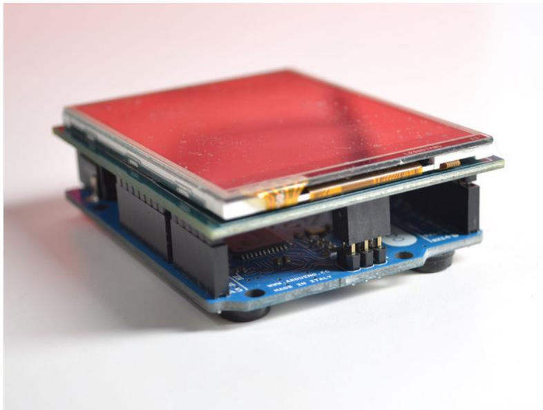
With this mod, the shield uses the ICSP header for data so make sure your duino (or stack of shields) has a ICSP plugged into the socket as above!
