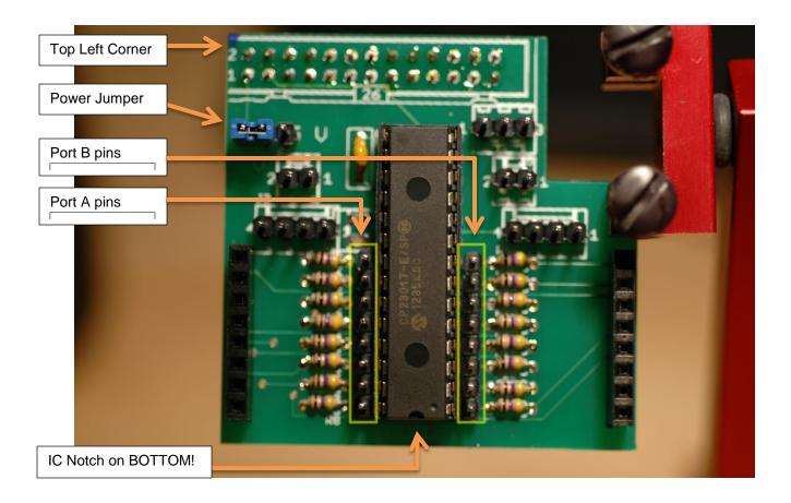
Take care to mount the socket and 23017 IC with notch pointed DOWN, not up.
