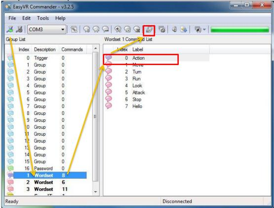
5. Once you are finished training and setting a command list click on "Generate Code..." save the \*.pde, load it in Arduino IDE or extract code from file.
