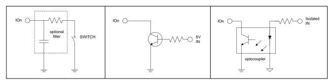
I/O pin connected to a switch (or switching sensor)
