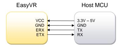
The initial configuration at power on is 9600 baud, 8 bit data, No parity, 1 bit stop. The baud rate can be changed later to operate in the range 9600 - 115200 baud.
