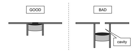
2. **No Obstructions, Large Hole** - The area in front of the microphone element must be kept clear of obstructions to avoid interference with recognition. The diameter of the hole in the housing in front of the microphone should be at least 5 mm. Any necessary plastic surface in front of the microphone should be as thin as possible, being no more than 0.7 mm, if possible.
