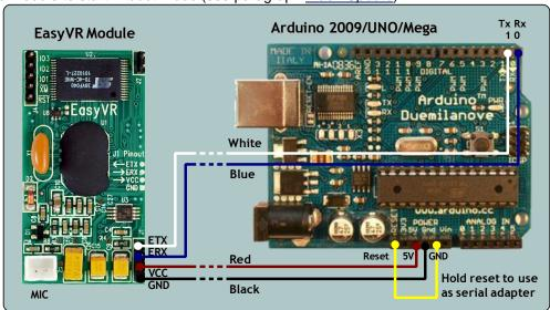
This configuration, with Reset shorted to GND, is for connection with the EasyVR Commander. To use the module from the Arduino microcontroller, you need to remove the short (yellow wire) and move the ETX/ERX
