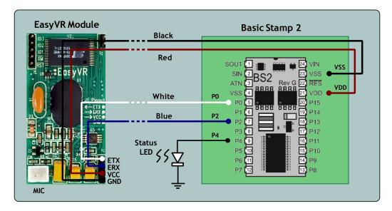
The status LED is used to signal that a recognition task is in progress and the application is listening for a voice command. This is optional and can be omitted.
