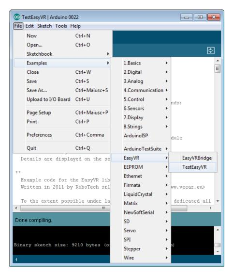
To test the EasyVR module with your Arduino programming IDE:
