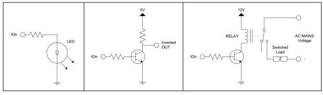
I/O pin directly driving a low-current LED
