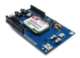
The 3G shield is based on SIM5216E module. The SIM5216 series is Multi-Band HSDPA/WCDMA/GSM/GPRS/EDGE module solution which supports HSDPA up to 3.6Mbps for downlink data transfer. The 3G shield can be used for 3G communication, it is controlled via AT commands and fully compatible with Arduino.
