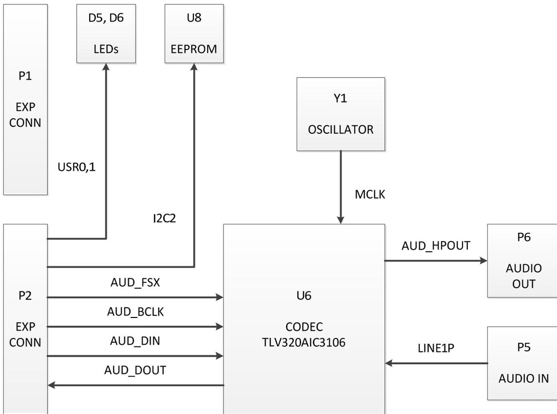
Figure 3. BeagleBone Audio Cape High Level Block Diagram
