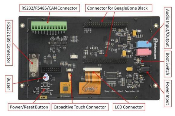
Figure 2. Back-Side View (Capacitive)
